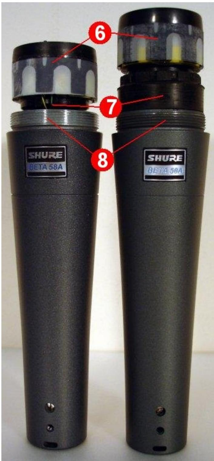
6) Although the microphone cells externally look similar the fake one sounds less defined than the original one. This is caused by the poor frequency range of the fake microphone. So if your brand new Shure microphone doesn't sound like it should this could be an indication that you have bought a fake one.
